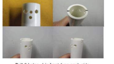
Drill 6 holes, 4 in front 1 on each side large enough for wire or connector
