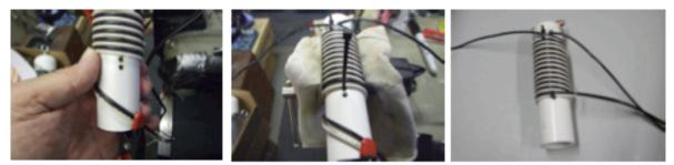
TAKE THE WIRE FROM THE RIGHT HOLE AND THE SAME COLOR WIRE FROM THE BOTTOM OF THE WRAPPED COIL AND CONNECT THEM TOGETHER - THESE WIRE WILL CONNECT TO THE CENTER OF THE S0239 CONNECTOR. TAKE THE EXTENDED WIRE ON THE UPPER LEFT AND JOIN IT TO THE WIRE OF OPPOSITE COLOR AT THE BOTTOM OF THE COIL WHICH WILL ATTACH TO THE GROUND OF THE S0239 CONNECTOR.
