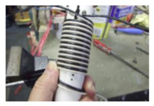
START WINDING THE WIRES TO THE RIGHT AROUND THE PVC PIPE KEEPING THE COILS TIGHT. AS IN THE PICTURES I COUNTED THE NUMBER OF TURNS OF BLACK WIRE -COUNT 12 TURNS DOWN. I PULLED BACK THE LAST WINDING AND DRILLED 2 HOLES FOR A PLASTIC TIE TO FASTEN THE LAST TURN.
