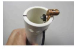
CUT AN 8 INCH SECTION OF #14 OR 12 GA. WIRE ATTACH WIRE TO RIGHT SIDE LUG BOLT LUG TO PVC USE ANY 2 COLORS
