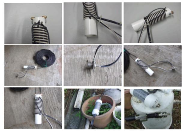
I TOOK THE COIL AND INCASED IT IN 2 INCH PLASTIC PIPE. I USED A DIFFERENT \$0239 CONNECTOR IN THE 2 IN. ENDCAP. I CUT A SLOT IN THE OTHER ENDCAP FOR THE WINDOW LADDER LINE TO COME IN AND FASTEN TO THE TWO COPPER LUGS. I USED DUCT SEAL COMPOUND TO SEAL THE ENDS AFTER FIRST USING ELECTRICAL TAPE AROUND THE CONNECTOR. THE PIPE LENGTH CAN BE TRIMMED. This is what I built - David N3GRH
