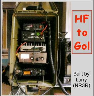
Complete HF station in a marine dry box. The station includes a Yaesu 817, a power supply, VHF 35-watt amp, keyer, mini antenna tuner, thru-box antenna connections, a compartment in the lid for accessories and more. *A perfect RACES HF station [ed]*!
